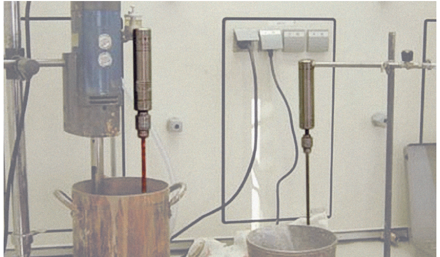
Compressed air stirrer PLR 12 with finger-operated oiler
